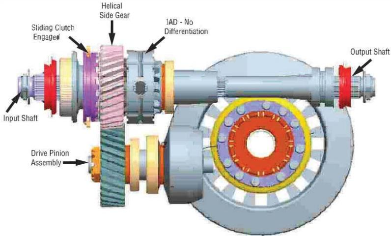
**The input shaft, helical side gear, IAD, and output shaft all turn at the same speed**
