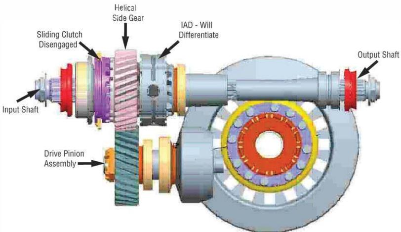
**The IAD will differentiate letting the output shaft turn at a different speed than the input shaft, helical side gear, and forward axle drive pinion**
