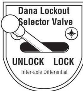
2. Momentarily let up on the accelerator to break engine torque. IAD lock will disengage.
