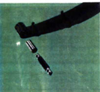
Threaded steel-to-steel pins and bushings in front springs last longer, eliminate side movement.
